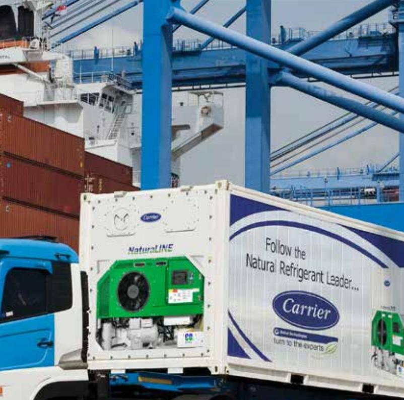
With a global warming potential of 1, the natural refrigerant carbon dioxide (CO<sub>2</sub>) provides a highly compelling case for environmental sustainability. To fulfill its potential for marine container applications, CO<sub>2</sub> refrigerant-based systems need to be highly efficient.
