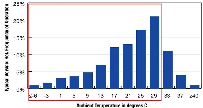
The majority of the time containers are in transit, ambient temperatures are below 31 degrees Celsius, where the NaturaLINE unit's efficiency is optimal for perishable loads. At ambient temperatures above 31 degrees Celsius, refrigeration performance is not affected, allowing the NaturaLINE unit to perform within the full operating envelope of a standard unit.
