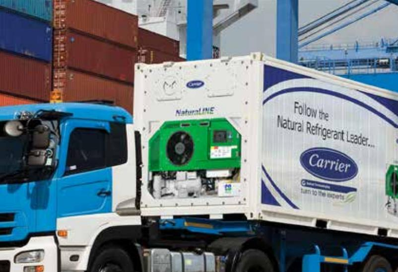
Natural refrigerant technology responds to the shipping industry's drive for sustainable refrigerated transport solutions. Among all the natural refrigerant alternatives, none presents a better solution for shipping lines than carbon dioxide (CO<sub>2</sub>), which is used in the NaturaLINE® container refrigeration system from Carrier Transicold.
