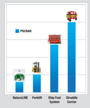
Operating pressures of a NaturaLINE system are a fraction of the pressures required by forklifts, straddle carriers, winches and watertight doors typically encountered by service personnel on ships and at depots.
