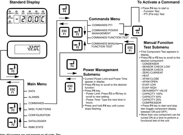
Note: All screens are *not* present on all units. The screens that display on the controller are determined by the Controller Software setting and the options installed on the unit.
