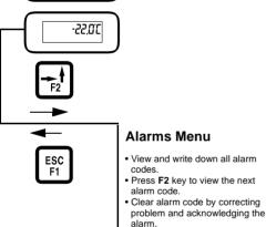
• To acknowledge an alarm, press F4 key with alarm code in display.
