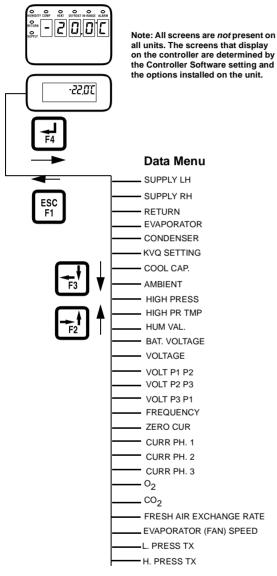
Figure 25: Data Menu Screen Flow Diagram
