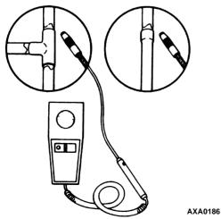
Figure 48: Test for Refrigerant Leaks
