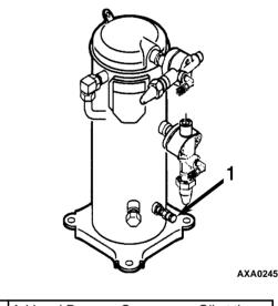
1. Add and Remove Compressor Oil at the Compressor Oil Fitting
