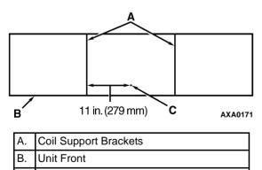
C. Insert Sensor at least 75 mm into coil between Tube Rows 2 and 3.
