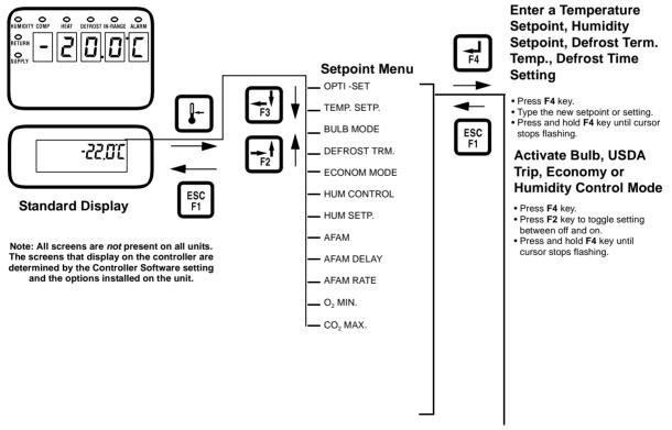
Figure 24: Setpoint Menu Screen Flow Diagram
