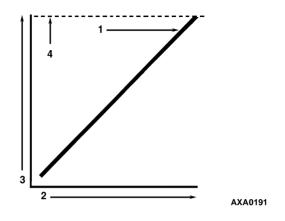
Close the vacuum valve and watch the movement of vacuum gauge needle. If needle continues to rise, this is an indication that a leak exists in the unit or connecting line. The leak must then be located and eliminated.
