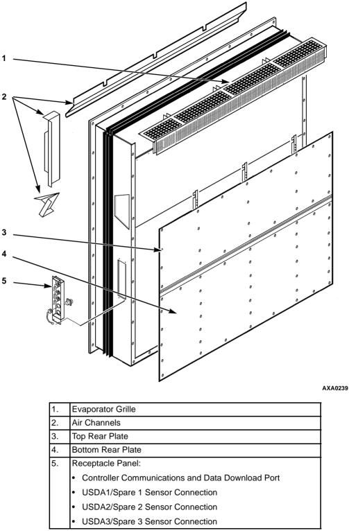
Figure 19: Unit Back View — Models with Heater Access Door (CSR20SL-144 , CSR40-145, CSR20SL-155 and CSR40SL-506)
