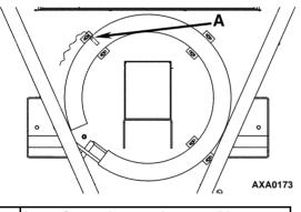
Insert Sensor into condenser coil between Tube Rows 1 and 2
