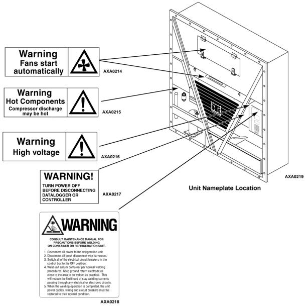
Figure 1: Nameplate and Warning Locations
