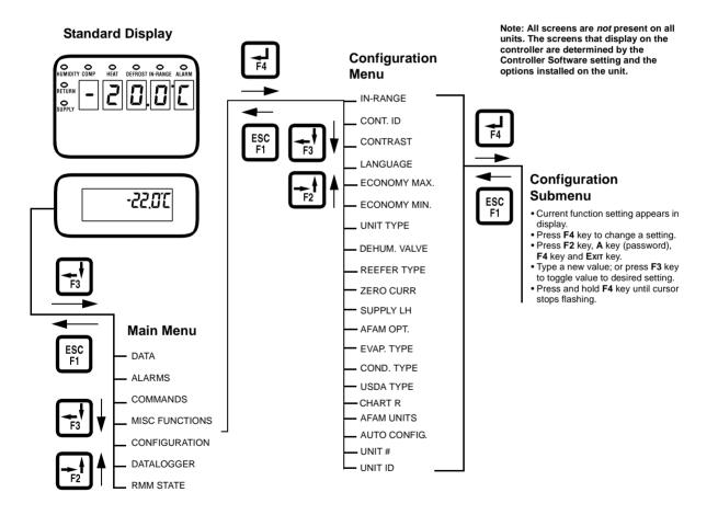
Figure 64: Configuration Menu Screen Flow Diagram
